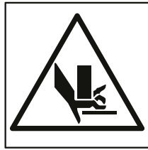
Risk of getting crushed - moving parts
